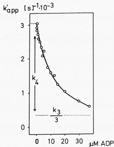
Fig. 3. ADP effect on the apparent first order rate constant of ATPase reaction. — No added phosphate. — A series of ATPase experiments has been performed using 16 different “inhibitory” ADP concentrations in the dark step. The chlorophyll content in this medium was adjusted to 25 \mu\text{g}/\text{ml} . When the light was switched off 0.2 \mu\text{M} gramicidin and 150 \mu\text{M} labelled ATP mixed with 0.1 to 50 \mu\text{M} ADP were added. The values of k_4 and k_3 can be estimated from this plot as indicated. The lower intersection with the y-axis normally gives k_3/1 + \text{ATP} \cdot K_m^{-1} ; but in our experiments ATP was twice the K_m value. From the data shown in this figure the following values were calculated: k_3 = 10^{-1} \text{ s}^{-1} and k_4 = 2.5 \times 10^{-3} \text{ s}^{-1} .
